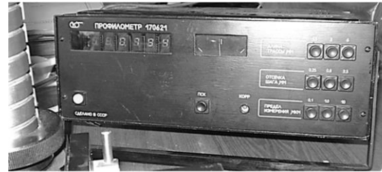
Fig. 10. Profilometer for measuring surface roughness: setting (a) and measuring part (b) Source: compiled by the author
