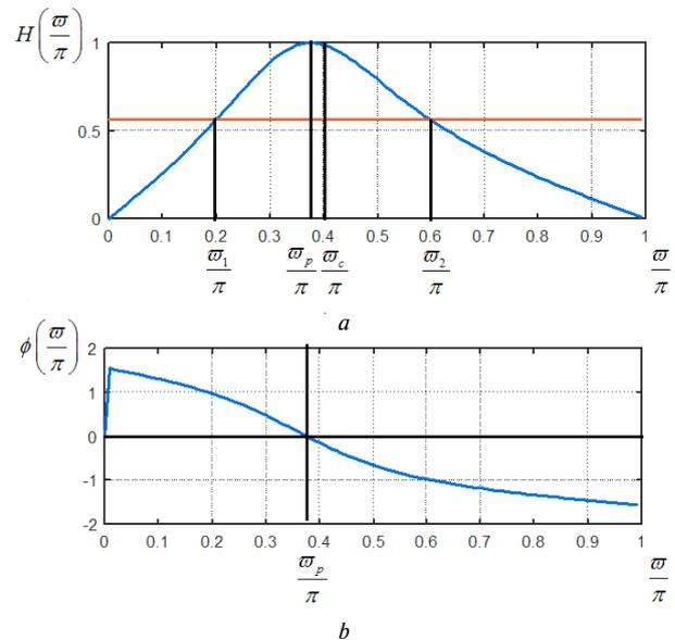
Fig. 3. AFR and PFR of a generalised normalised digital bandpass filter at oscillation  $RP = 5$  and cut-off frequencies:
