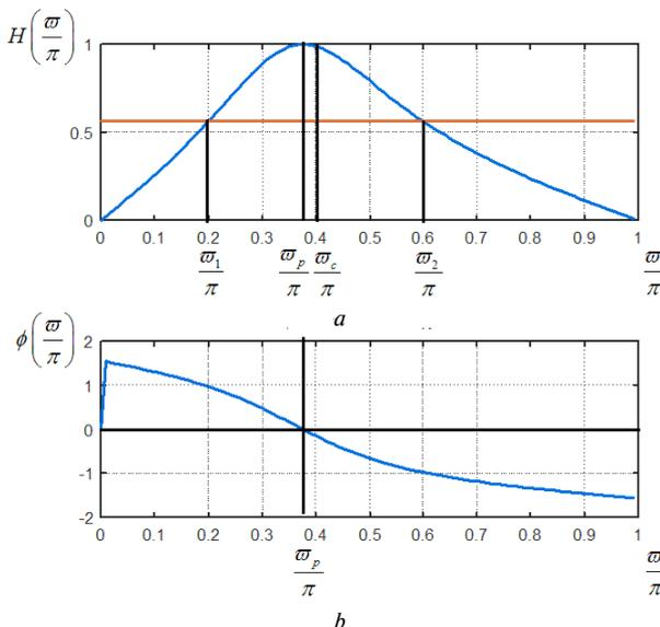
Fig. 4. AFR and PFR of a generalised normalised digital band-pass filter at oscillation  $RP = 5$  and cut-off frequencies:
