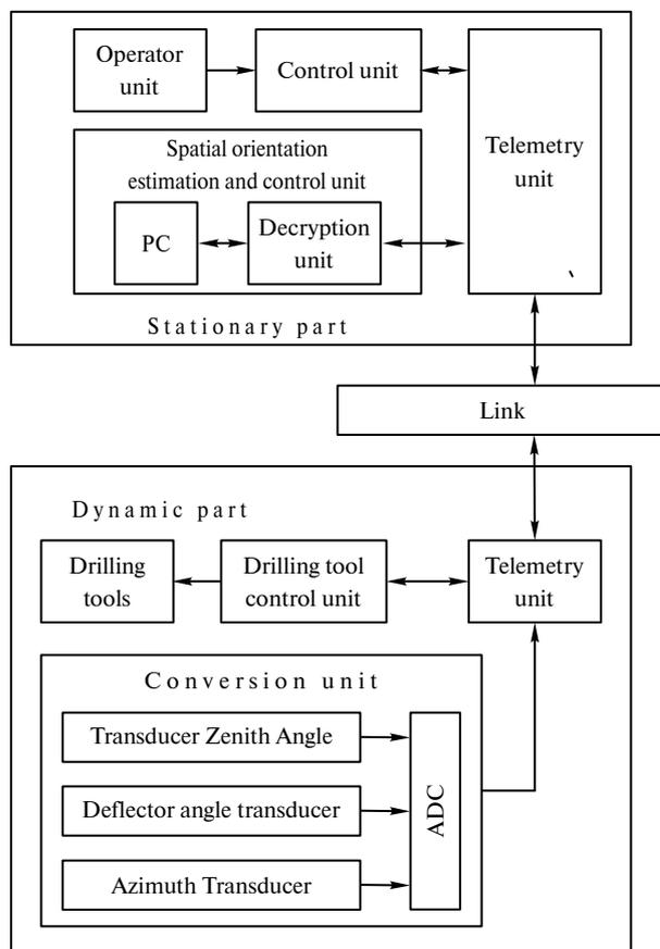
Fig. 1. Structure diagram of a computerised spatial orientation control system (CSOCS) for drilling facilities
