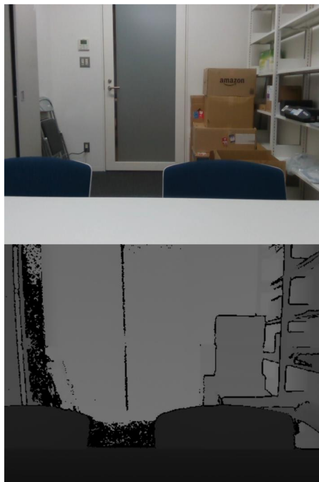
Fig. 1. Color image and depth map, obtained with structured light sensor
