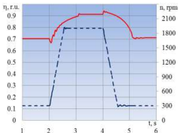
Figure 2. Characteristics of a rotational speed (---) and efficiency (-) of baseline motor for the third design task
