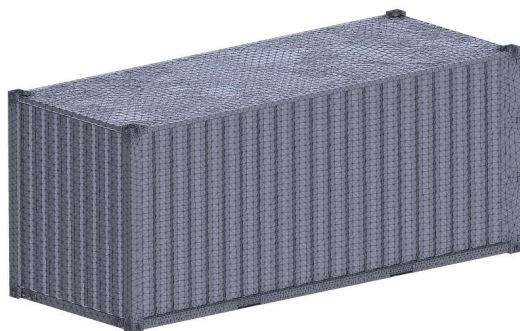
Fig. 7. Finite element model of a container
