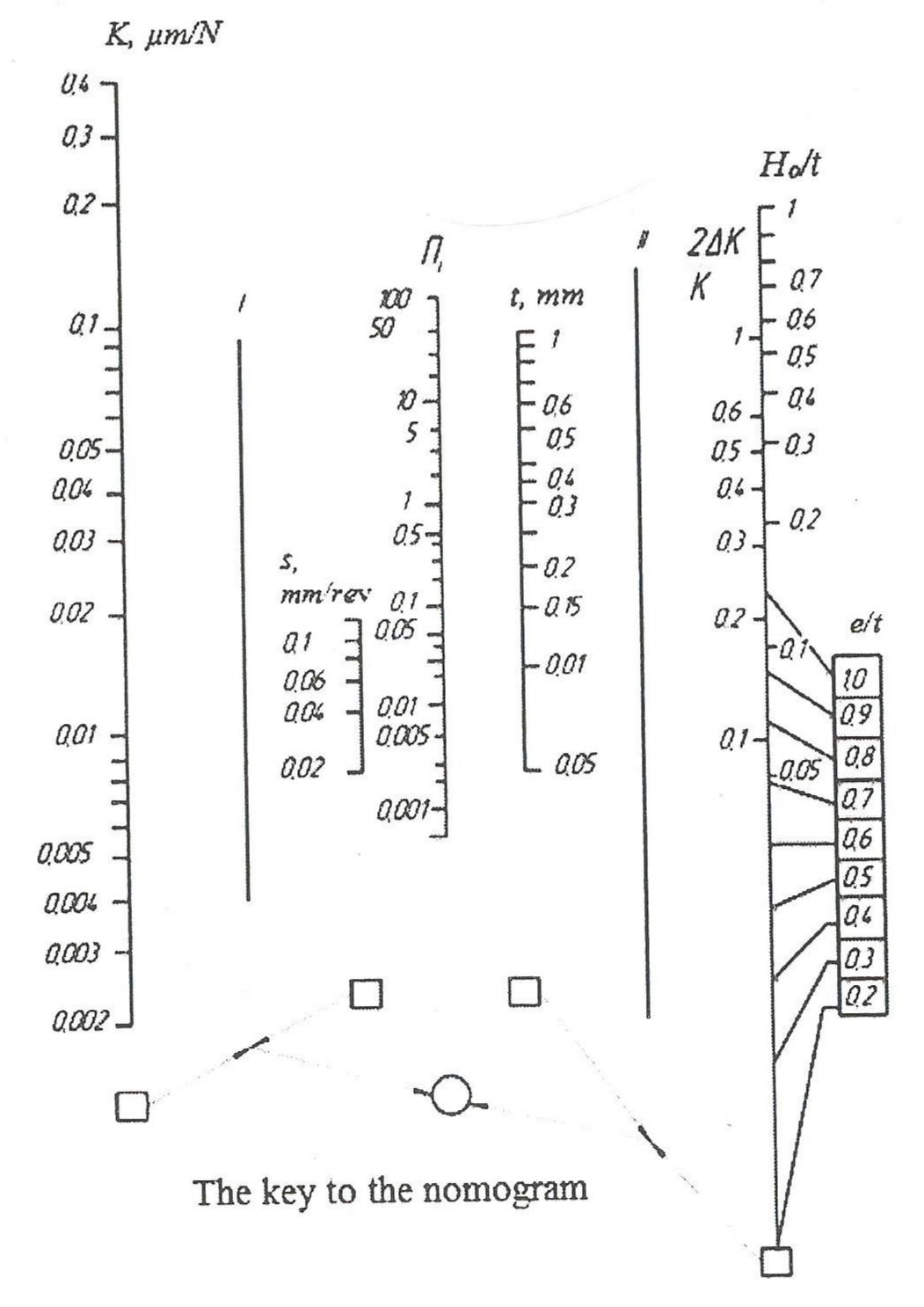
**Fig. 1.** Determination of static errors in the boring of samples (steel 35) according to the nomogram: O – values of the individual errors  $\Pi_i$ ; K – the elastic system compliance; S – feed per revolution; t – cutting depth
