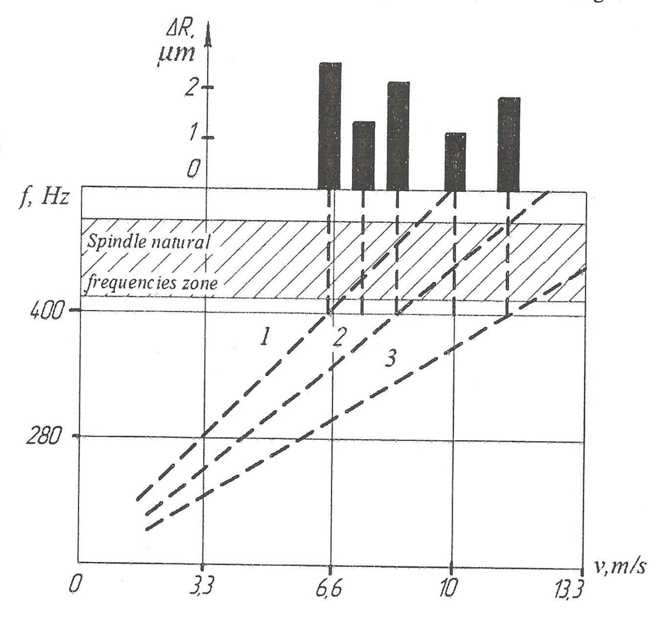
Fig. 3. Dependencies of deviations from roundness when you change the frequency of the idle rotation of the spindle 1, 2, 3 – harmonics of vibration excitation caused by the ball-bearings at idle rotation
