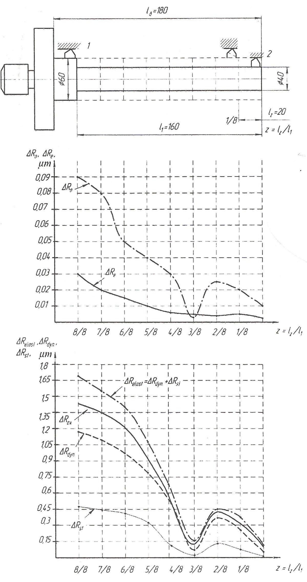
Fig. 2. The dependence of the static and dynamic errors on the ratio of the lengths of two-stepped boring bar (Steel 35  $t = 0, 2 \, \text{mm}$ ,  $s = 0, 05 \, \text{mm}$  / rev,  $v = 3, 3 \, \text{m}$  / c)
