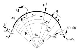
Fig. 1. Calculation scheme of the circular arch
