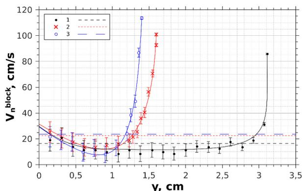
**Fig. 3.** Distribution of the normal component of the local flame speeds along the torch for: 1)  $\alpha=0.93$ ; 2)  $\alpha=1.3$ ; 3)  $\alpha=1.38$ . The dashed lines mark the corresponding average values  $\langle V^n \rangle$ : 1 – 13.6 cm/s; 2 – 22.6 cm/s; 3 – 23.6 cm/s.
