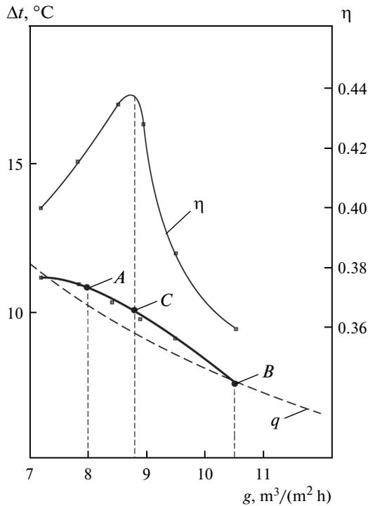
Fig. 2. Difference between the water temperatures at the cooling tower inlet and outlet  $\Delta t$  and mechanical-draft cooling tower efficiency factor  $\eta$  ( $S_{cool} = 2 \times 192 \text{ m}^2$ ) vs. the specific hydraulic load.
