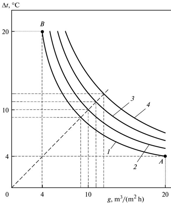
Fig. 1. Hyperbolic curves of a constant heat load,  $q$ , MJ/(m<sup>2</sup> h): (1) 335, (2) 419, (3) 502, and (4) 603.
