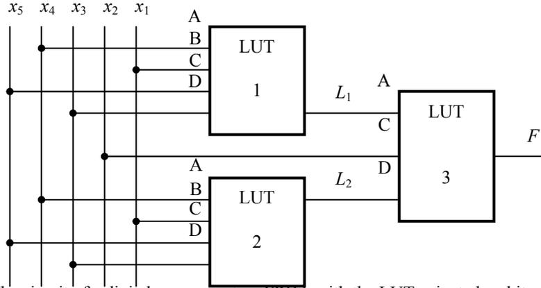
**Fig. 1** The circuit of a digital component on FPGA with the LUT-oriented architecture
