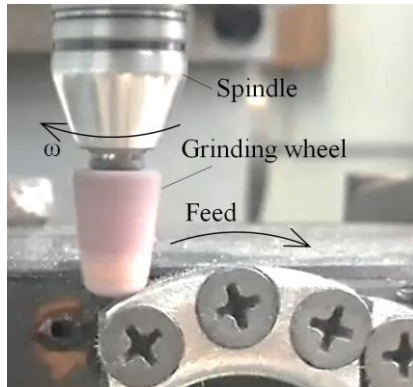
Fig. 12. Contour grinding with infinitesimal tool pressure (nanotechnology)
