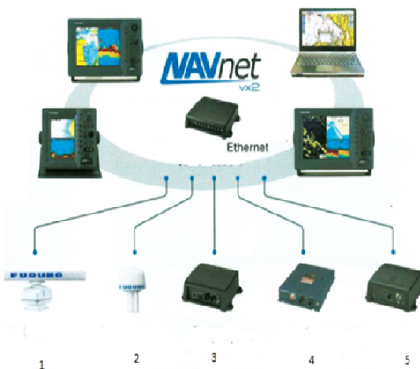
Fig. 1. Marine integrated navigation system
