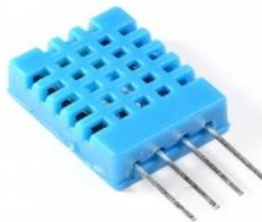
Fig. 5 – Temperature and humidity sensor DHT11
