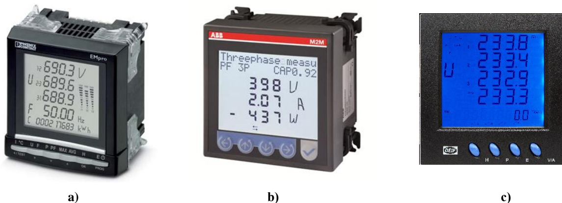
Figure 1 - a) EEM-MA600, Phoenix Contact; b) M2M, ABB; c) MIC, DEIF;
