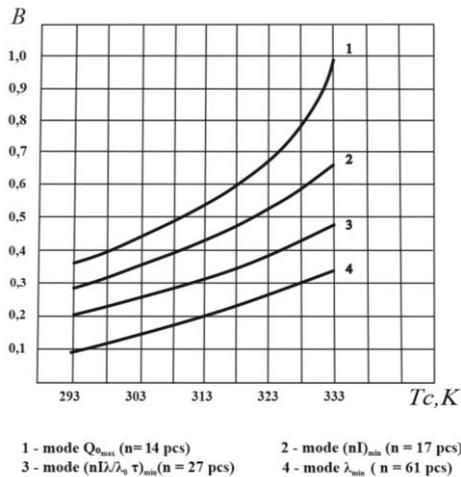
**Fig. 1. Relative operating current  $B$  vs medium temperature  $T_c$  for various initial characteristic current operating conditions at  $T_c = 338\text{K}$  at**
