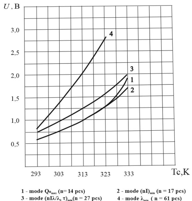
**Fig. 4. Dependence of voltage drop  $U$  on medium temperature  $T_c$  for different initial characteristic current operating modes at  $T_c = 338\text{K}$  at**
