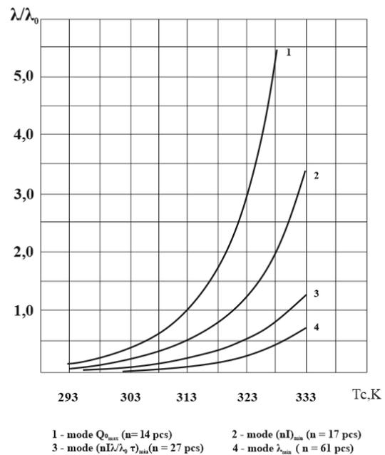
**Fig. 9. Relative failure rate  $\lambda/\lambda_0$  dependence on medium temperature  $T_c$  for different initial characteristic current modes at  $T_c = 338K$  at  $T_0 = 293K$ ;  $l/S = 4.5$ ;  $Q_0 = 0.5W$ ;  $t = 10^4 h$**
