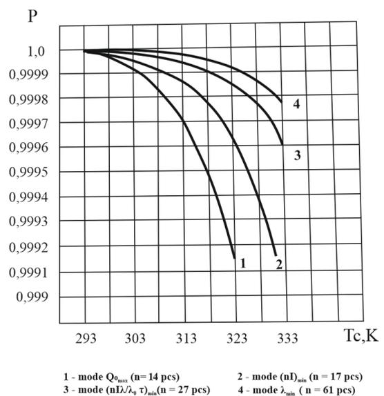
**Fig. 10. Failure probability  $P$  dependence on medium temperature  $T_c$  for different initial characteristic current operation modes at  $T_c = 338K$  at  $T_0 = 293K$ ;  $l/S = 4.5$ ;  $Q_0 = 0.5W$ ;
