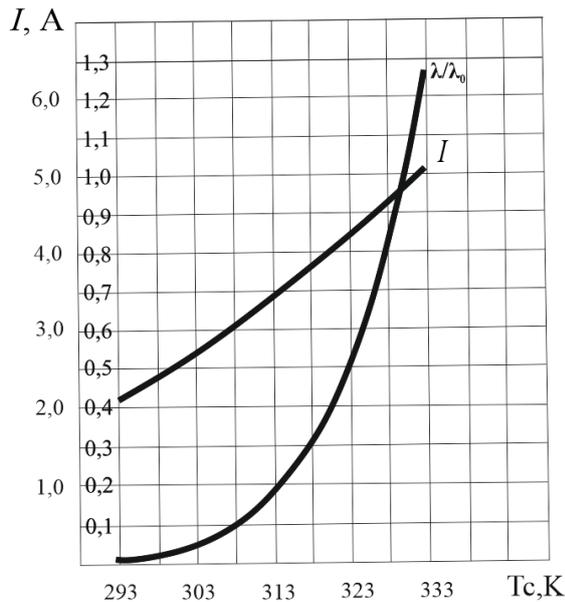
Fig. 11. Dependence of operating current  $I$ , relative failure rate  $\lambda/\lambda_0$  on medium temperature  $T_c$  for different initial characteristic current operating modes at  $T_c = 338\text{K}$  at
