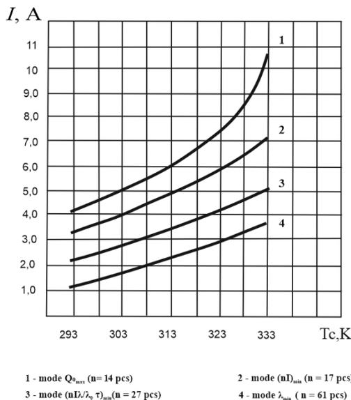
**Fig. 2. Dependence of operating current  $I$  magnitude on medium temperature  $T_c$  for different initial characteristic current operation modes at  $T_c = 338\text{K}$  at  $T_0 = 293\text{K}$ ;  $I/S = 4.5$ ;**
