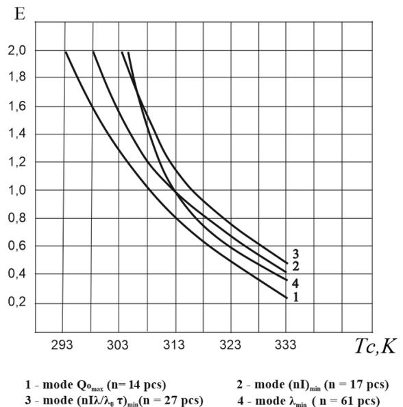
**Fig. 3. Dependence of refrigerating factor  $E$  on medium temperature  $T_c$  for different initial characteristic current operating conditions at  $T_c = 338\text{K}$  at  $T_0 = 293\text{K}$ ;  $I/S = 4.5$ ;  $Q_0 = 0.5\text{W}$**
