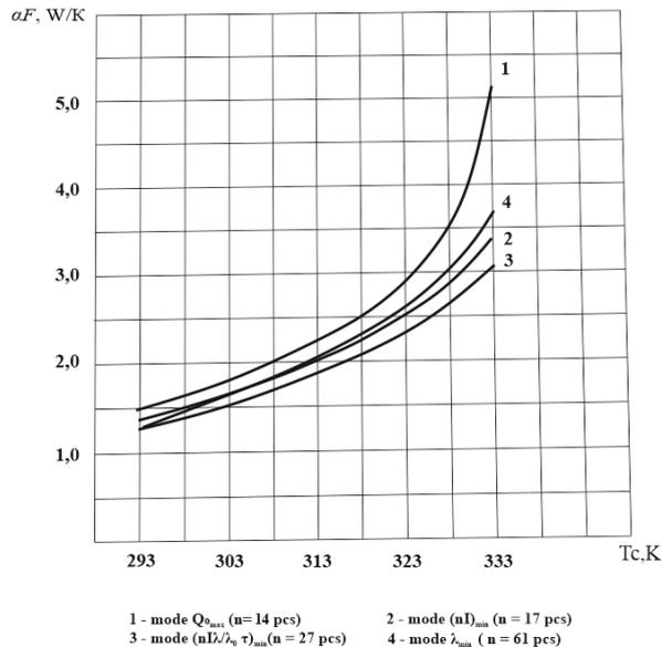
**Fig. 8. Dependence of the required heat dissipation capacity  $\alpha F$  of the heat sink on the medium temperature  $T_c$  for different initial characteristic current operation modes at  $T_c = 338K$  at  $T_0 = 293K$ ;  $l/S = 4.5$ ;  $Q_0 = 0.5W$ ;
