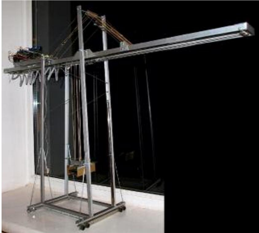
Fig. 7. Photograph of the experimental setup of the container crane.
