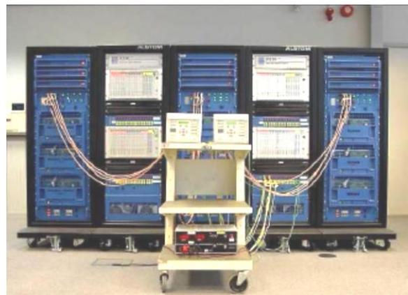
**Fig. 6. Apparatus-program test complex RTDS.**
