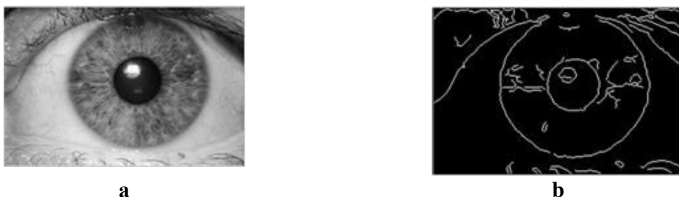
Fig. 1. Canny edge detection results: a – input image; b – binary representation of the edges
