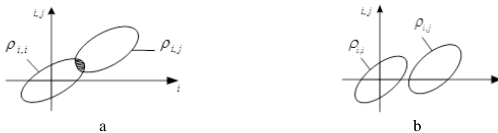
Fig. 1. Areas of distribution of two-dimensional quantities \rho_{i,i} , \rho_{i,j} : a – situation with higher accuracy of parameter estimates \Delta \hat{\rho}_i ; b – situation with higher distinguish ability of subschemes S_i , S_j .
