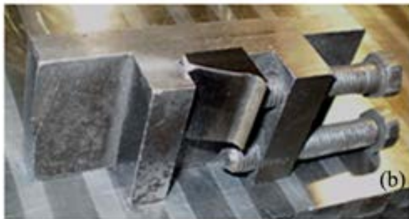
Fig. 11. Samples prepared from fragment teeth when the sample is clamped in the fixture (a) and installed onto the machine table (b)
