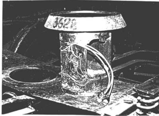
Figure 2 – Force transducer for three orthogonal directions
