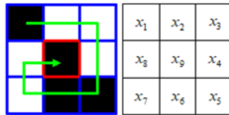
Fig.3. Cells’ location: red – current cell; blue – neighbors, cells’ numeration is going through green arrow Source: compiled by the author
