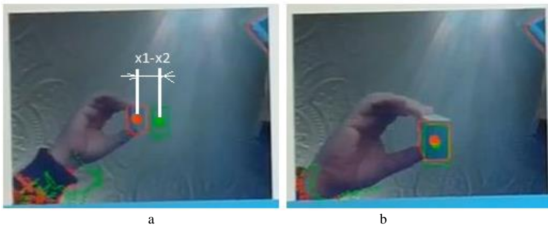
Fig. 3. Dependence of the difference in positions of the center of mass of objects on the distance: a – upon moving objects away; b – upon moving objects in Source: compiled by the authors
