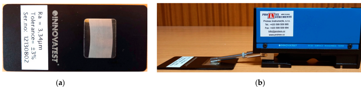
Figure 4. (a) Specimen measured to determine roughness parameters; (b) R130 roughness tester at work.
