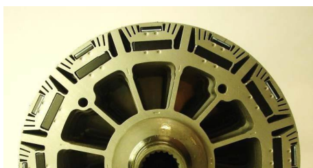
Fig. 5. The rotor of BMW i3, D_{or}=180 mm, p=6
