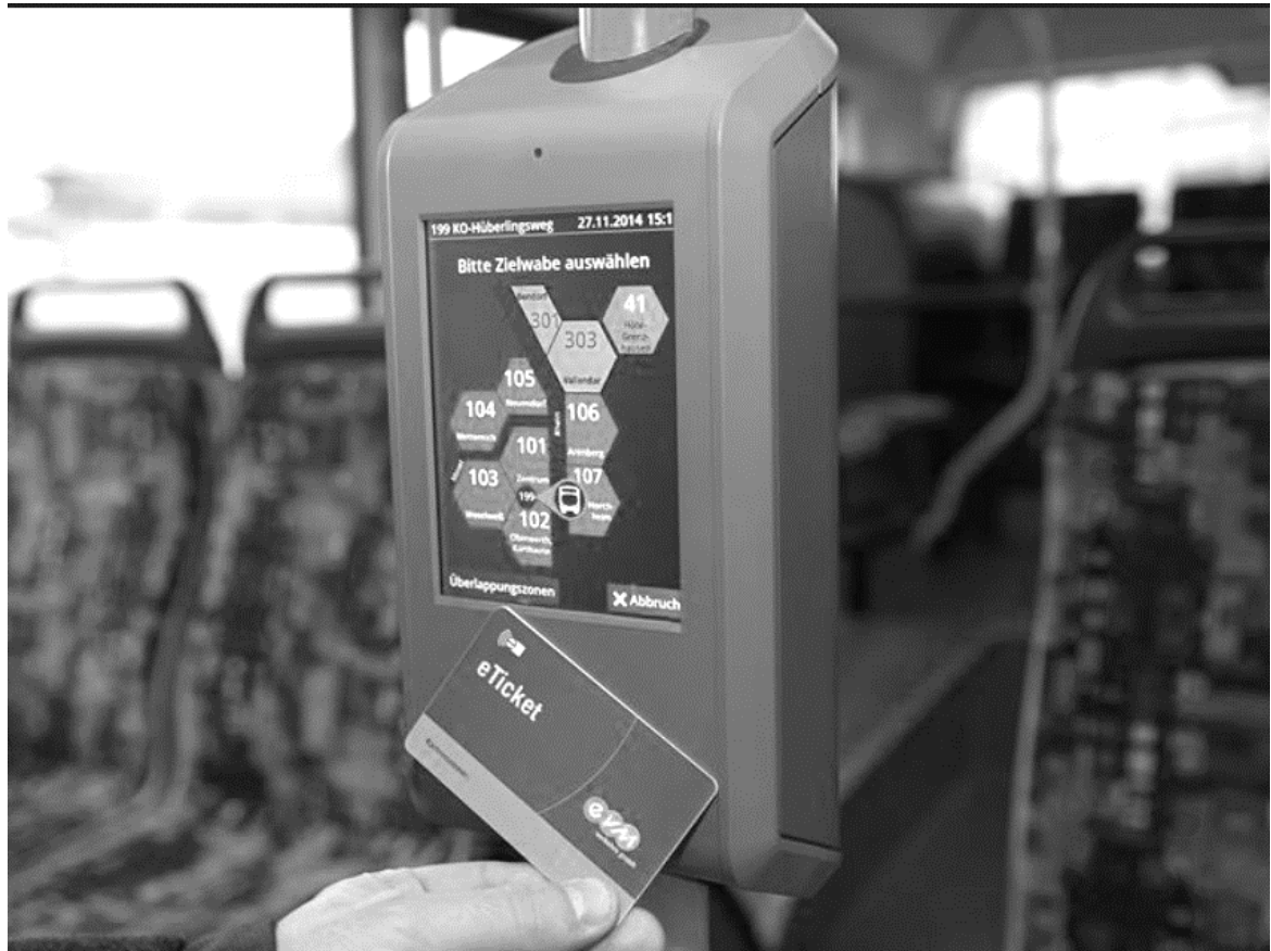
Figure 1.10. Example of a validator for the e-ticket system [71]
