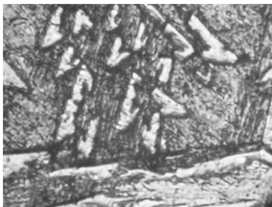
Fig. 1. Microstructure of VT3-1 titanium alloy after quenching; \times 200
