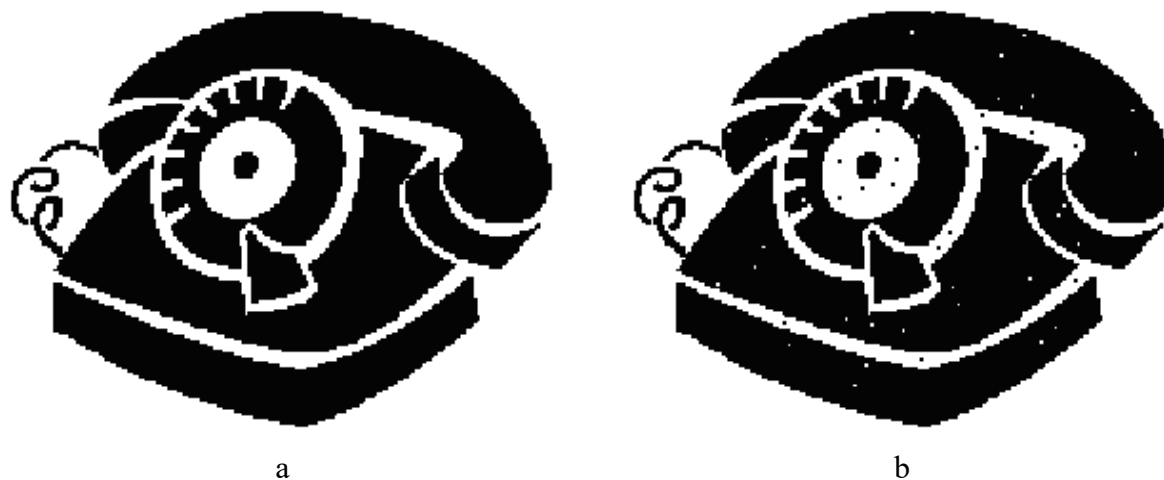
Fig. 1. The result of embedding of additional information into binary digital image: a – digital image-container; b – digital image-stego
